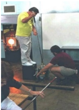
Figure (8) Blow-shaping with rotation
