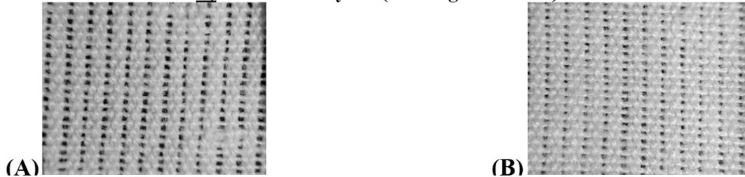
Fig. (8) Illustration of the pore size for produced fabrics: A) sample 7 produced from 50% banana: 50% cotton (high porosity), B) sample 1 produced from 25% banana: 75% cotton (low porosity)
