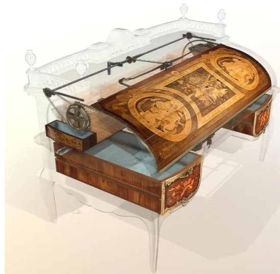
Fig (14) The opening mechanism of the rebuilt desk. Toothed poles are inserted on both sides of the desk and connected by a central axis
